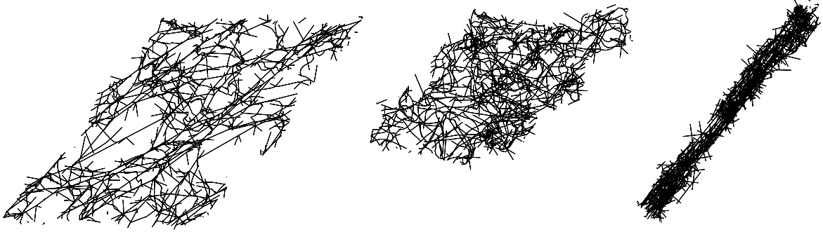
Figure 4.6: Left: U_1 = U_2 = 0 , middle: F_1 = F_2 = 0 , right: F_1 = 0 U_2 = 0 . The snapshots are properly scaled and taken under an applied shear strain \Gamma = 0.8 . The left network has dimensions 40 \times 40 \mu\text{m} .
